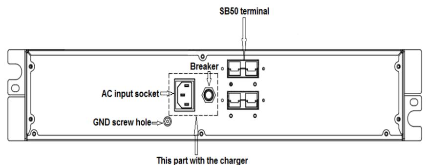
Fig.8 Battery pack rear panel
